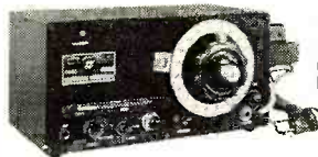
LAMPKIN 205-A FM MODULATION METER Indicates peak voice deviation, ± 25 KC. Tunes 25-500 MC. in one band. Speaker. Oscilloscope output. Relative field-strength meter. Weight 13 lbs. Width 12". Price $240.00 net.
