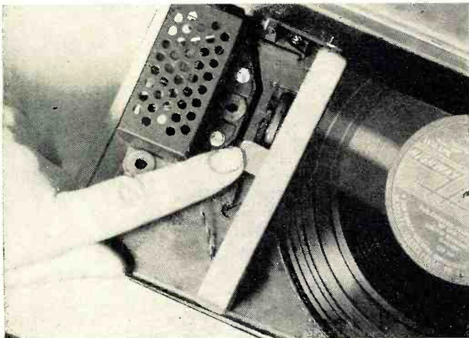
Fig. 2. Pressing the small tab on the tone arm, shown here, releases the tone arm. Moving it to the right starts turntable.
