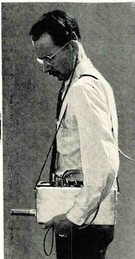
Fig. 1. The counter in use. Note the bone-conduction headset, carrying strap, and the position of the unit's carrying handle.
